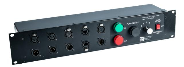
Lawrence is a rack-mount XLR continuity tester designed for high-volume cable testing needs, such as returned cable cases in rental shops. As a pass/fail tester, Lawrence doesn't evaluate what's wrong with the cable; he just quickly determines whether it's wired correctly, without any open, shorted or crossed conductors, so it can be sent to the repair shop if needed.
