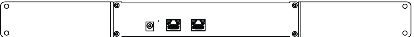
Back panel includes: (2) Ethernet; 5VDC/2A input
